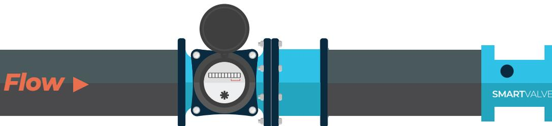
Install after water meter and before pressure reducer or booster pump. Soon after the backflow is usually good place.
