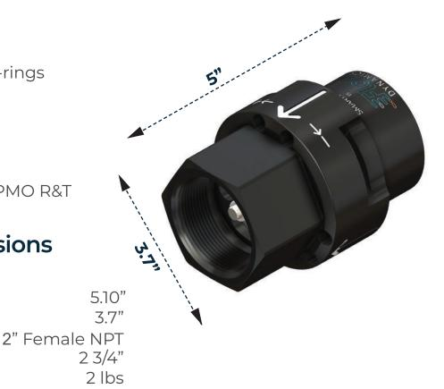
For best results install the Smart Valve downstream of water meter and backflow preventer (if present), but before any other valves or equipment such as a pressure reducer or booster pump. Where possible it is recommended (but not critical) to have 10 diameters of straight pipe before and after the valve. All threaded installations require pipe tape.
